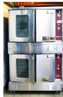
Commercial Convection Oven, natural gas, 45 meals per unit, requires hood, cooking time = 30 minutes
